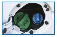
DEF's effects on the fuel supply system are common to that of water. Having DEF enter the fuel system can lead to high pressure fuel pump and injector wear, rust, corrosion, pitting, distortion of materials, plugged fuel return lines and may exhibit the following symptoms;
