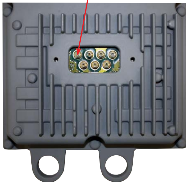
7 Screw Style (Early) Place positive lead on this screw
