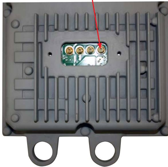
4 Screw Style (Late) Place positive lead on this screw
