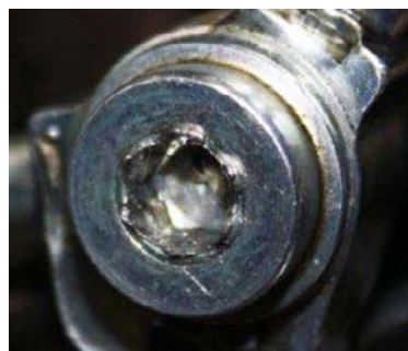
Damaged Banjo Bolt
